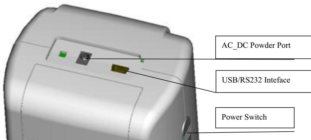
Figure 3 Interface Diagram
