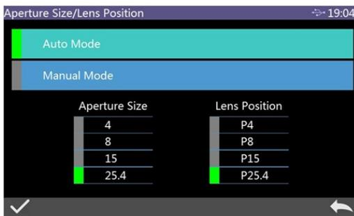
Figure 12 Measuring Aperture / Lens Position Selected Interface
