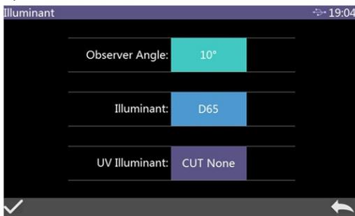
Figure 13 Light Source Setting Interface
