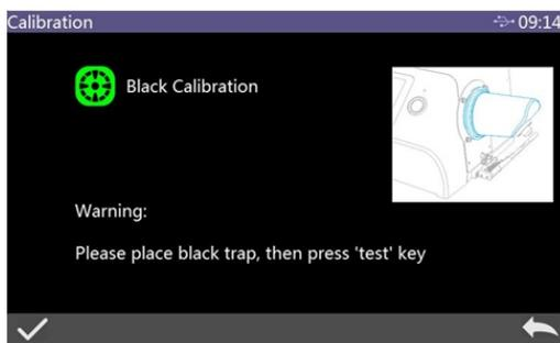
Figure 5 Reflective Black Calibration Interface
