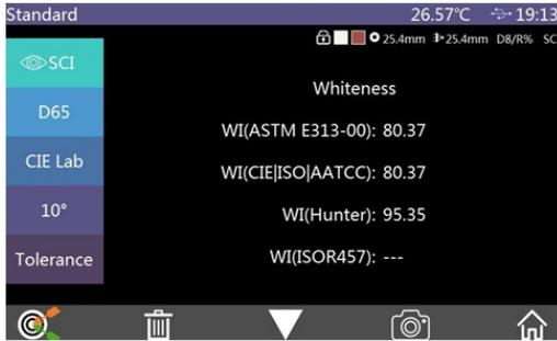
Figure 41 Whiteness Display Interface Under Standard Measurement
