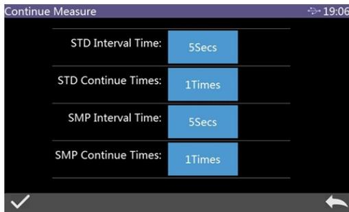
Figure 18 Continuous Measurement Mode Setting Interface
