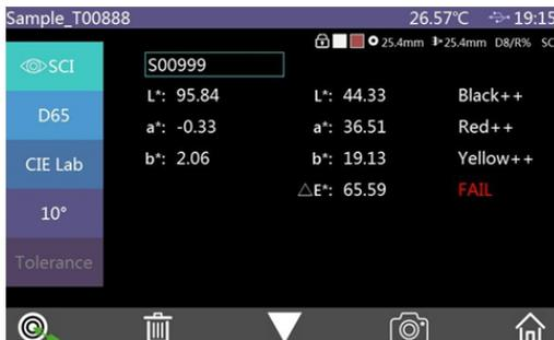
Figure 47 Sample Measurement Interface Under Absolute Value Mode
